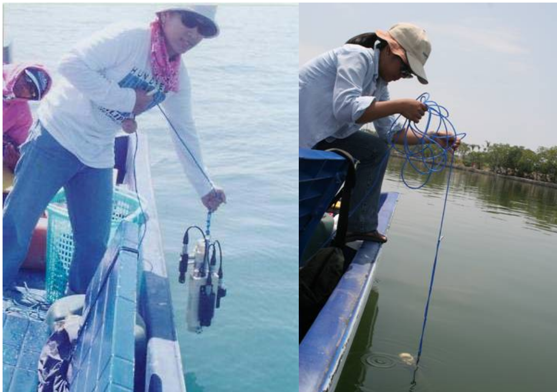
Figure 10. Sampling with the CTDO-probe.
