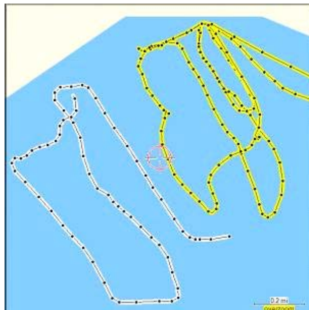
Figure 18. Illustration of the boat tracking recorded with a GPS to estimate the surface of the area of fish cages in an area.
