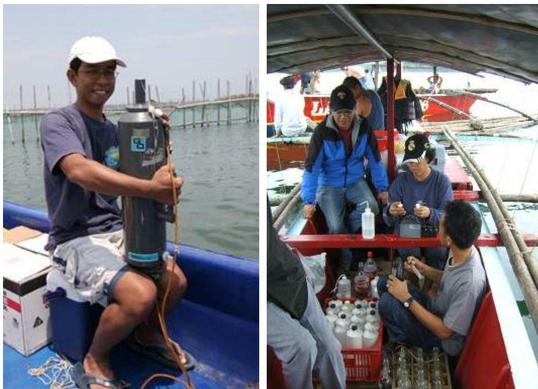
Figure 12. Left: Water samples taken with a Niskin water sampler in Bolinao Bay. Water sampling in Taal Lake.
