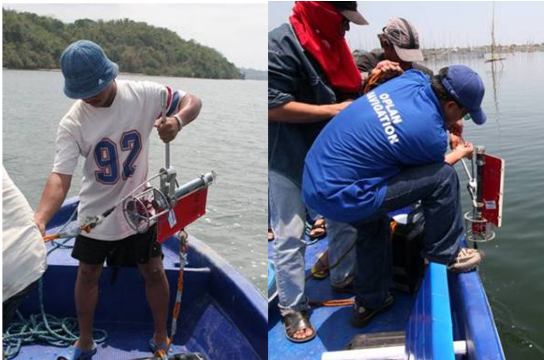
Figure 7. Deploying current meters.
