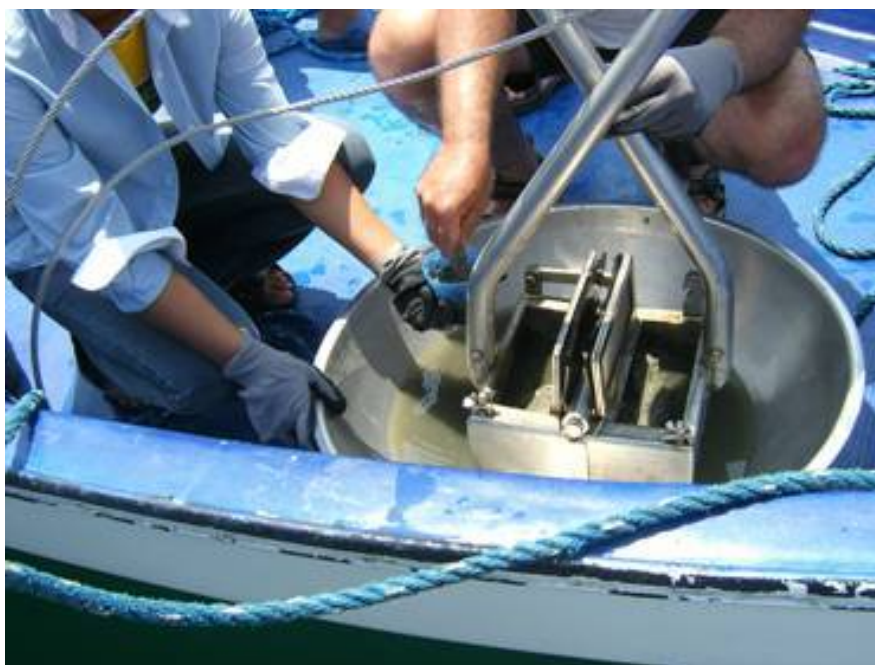
Figure 14. The grab sample is inspected through the lid on top of the grab. A sample for chemical analysis is taken from the upper surface (2 cm).
