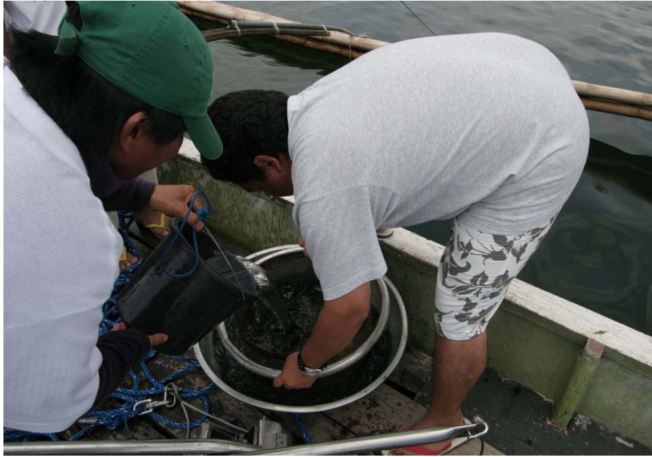
Figure 15. Biological samples gently sieved through a 1mm round hole sieve immersed in sea water.
