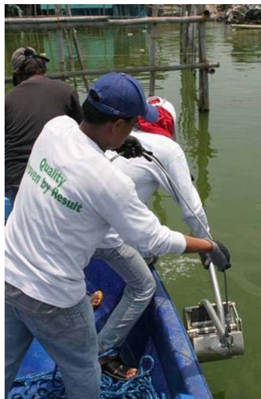
Figure 13. Illustration of the van Veen grab and picture of lowering the grab into the water.
