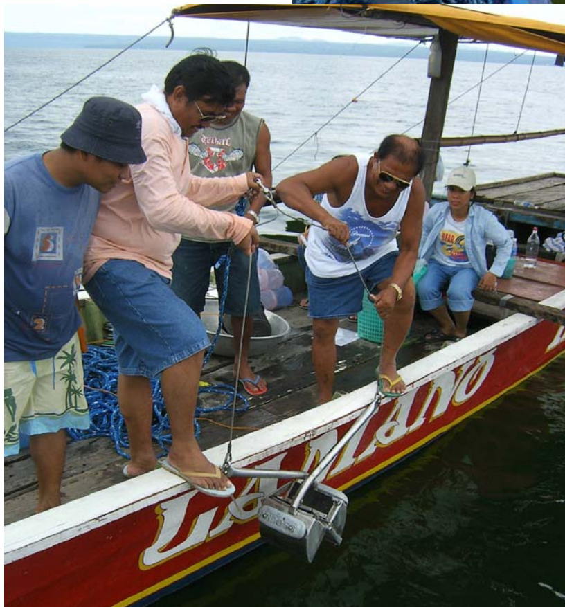
Figure 17. Illustration of the van Veen grab and picture of lowering the grab into the water.
