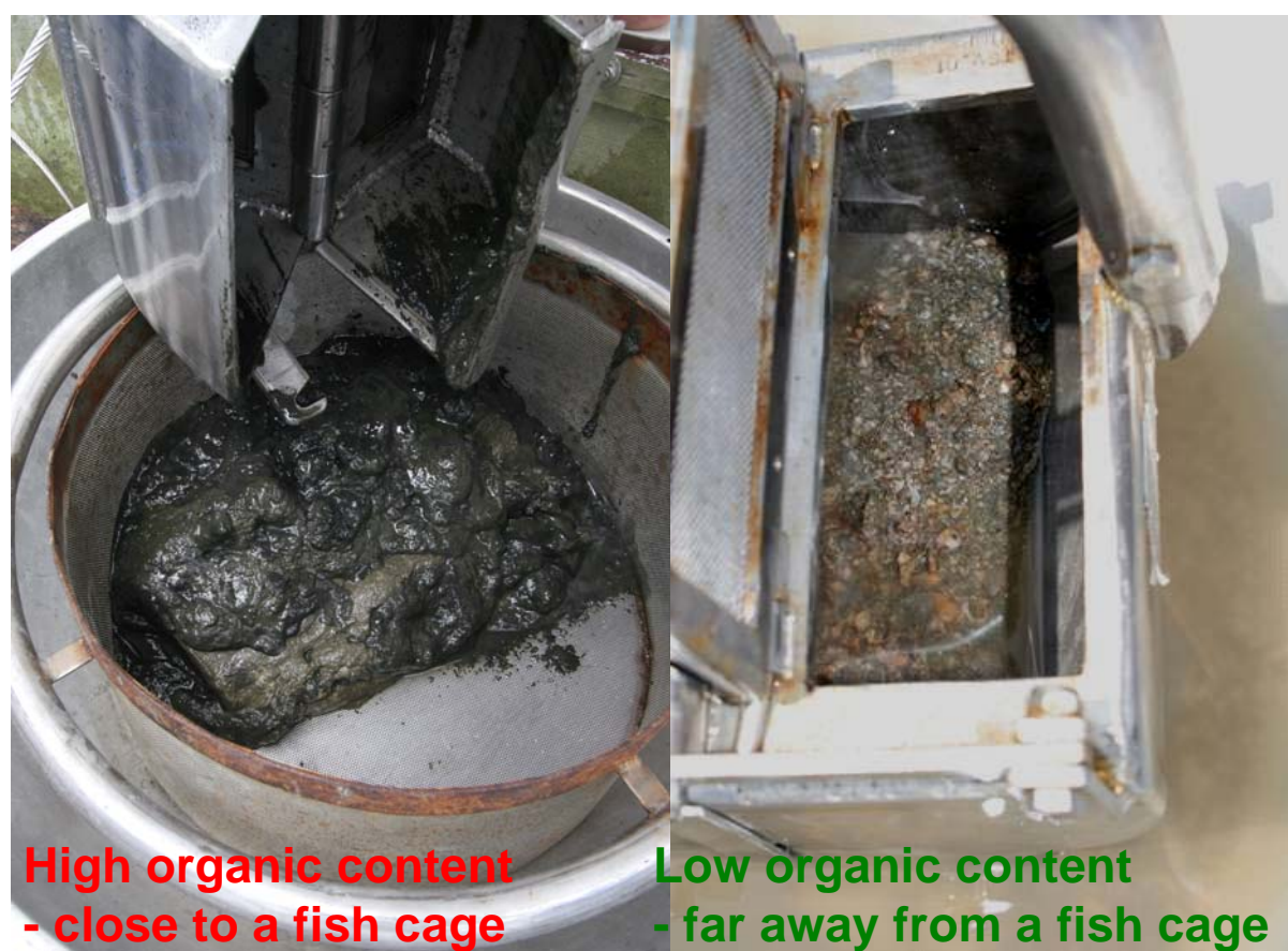
Figure 20. Sediment samples from sites with different environmental conditions. The left picture is of sediments close to a fish cage; the sediments have high organic content, no live animals and smelling H_2S . Right picture is from an area far away from a fish cage; where the sediment is in good conditions (picture is not from Taal Lake but used as an illustration of “very good” sediment conditions).
