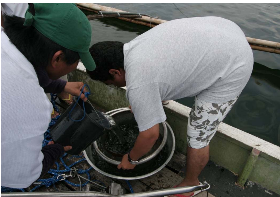
Figure 19. Biological samples gently sieved through a 1mm round hole sieve immersed in sea water
