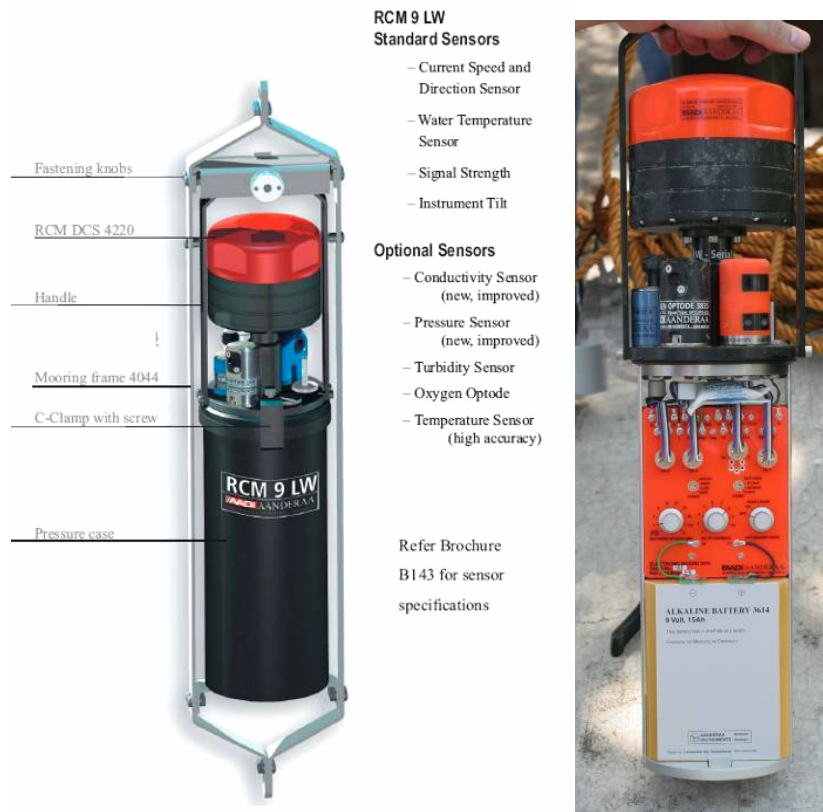
Figure 4. Aanderaa RCM 9 LW current meters equipped with sensors for measuring conductivity, turbidity, oxygen and pressure (depth).
