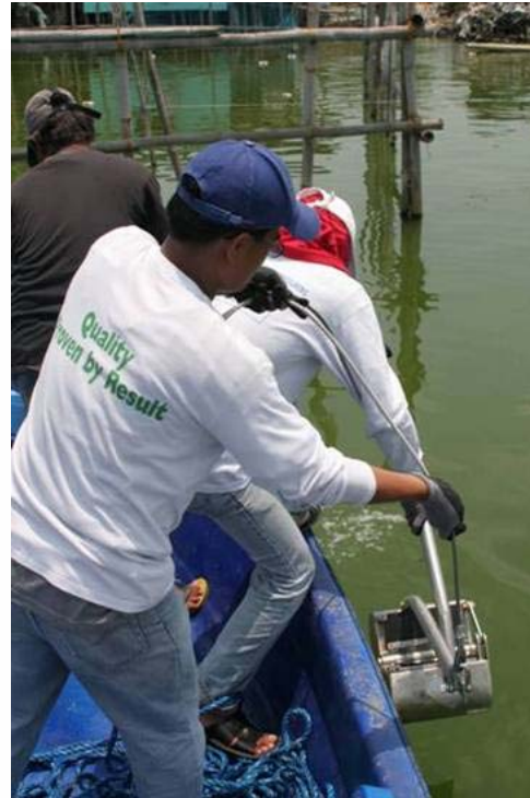
Figure 20. Illustration of the van Veen grab and picture of lowering the grab into the water.
