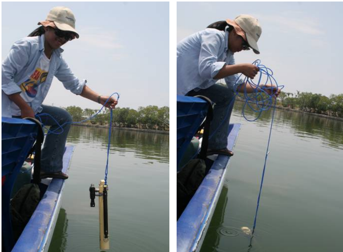
Figure 16. Sampling with the CTDO-probe.
