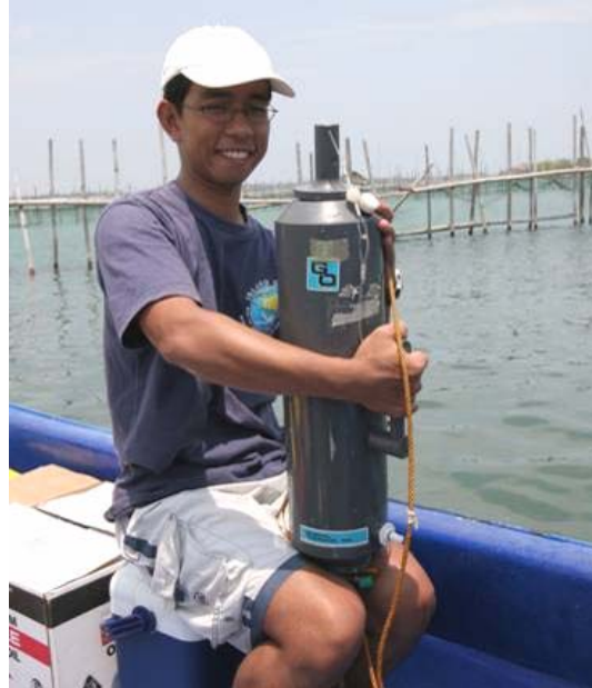
Figure 12. Niskin water sampler was used for collecting the water samples.
