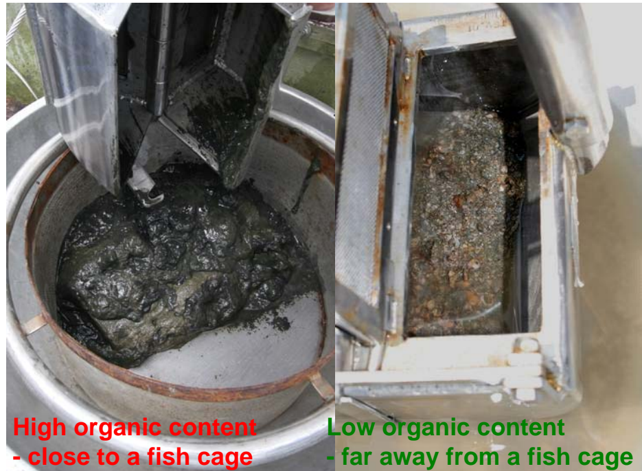
Figure 23. Sediment samples from sites with different environmental conditions. The left picture is of sediments close to a fish cage; the sediments have high organic content, no live animals and smelling H_2S . Right picture is from an area far away from a fish cage; where the sediment is in good conditions.
