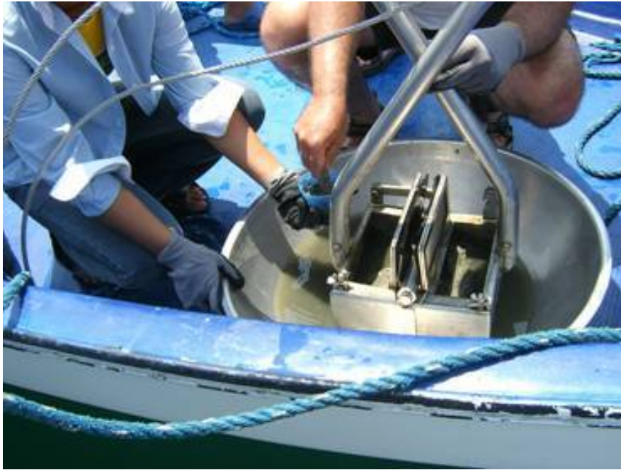
Figure 21. Sediment sample inspected Samples for chemical analysis taken from the upper 2 cm surface.
