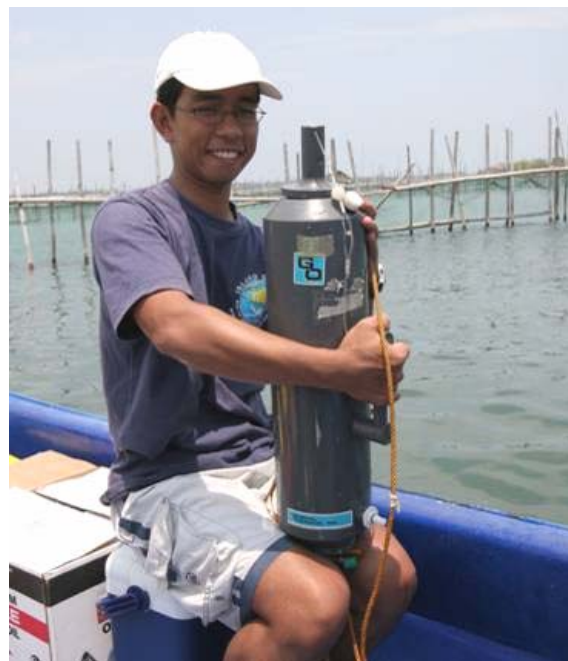
Figure 14. Niskin water sampler was used for collecting the water samples.
