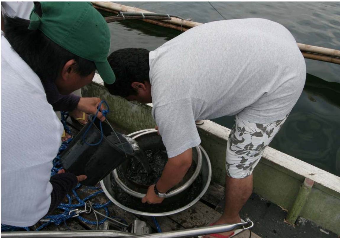
Figure 22. Biological samples gently sieved through a 1mm round hole sieve immersed in sea water
