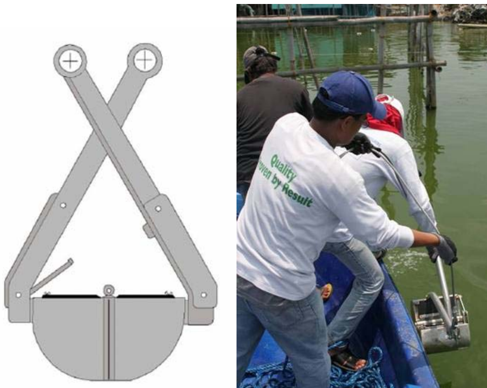
Figure 20. Illustration of the van Veen grab and picture of lowering the grab into the water.
