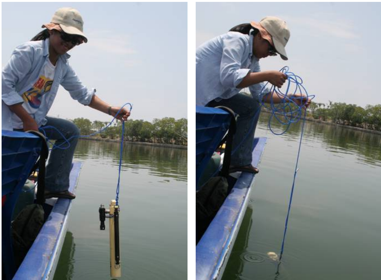
Figure 16. Sampling with the CTDO-probe.
